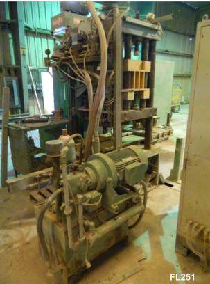
Hydraulic Press for making trim tiles. Extruded clay slug is placed on the table which is then automatically slid into place and pressed and table is then returned to loading position. Powered by a GEC Machines 15kw hydraulic power unit. Size:DE160L/4 No. 84129892
