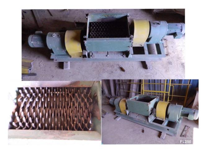
Double shaft green waste clay chopper with two counter rotating 5.5kw gearmotor drives. Used to reduce the size of green extruded clay waste for re-use. Diameter of roller is 300mm. Usuable roller length is 650 mm. Width of gap is 5mm. Commissioned in 1985.
