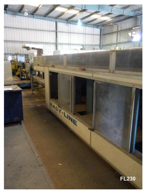
Automated sorting and packaging line for ceramic tiles. With operator station for visually checking for imperfections and DICO PLANAR automatically checking for flatness and sizing based on input specifications. Stacks the tiles in multiple stackers after inspection so that they may be packaged automatically in a wrap-around carton.
