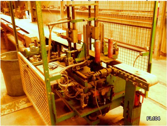
Can cut clay column up to 4.25" wide and 13" high with a self cleaning wire. Maximum cut length is 13 inches. Cuts per minute are 50 for 8" length (35 for 13" length). Cuts are controlled electronically with encoded DC drive. Electric control panel included. Pneumatic pre-grooving for products such as split tile. Commissioned in 1996. Asking \$17,500 (original price DM 131,500).
