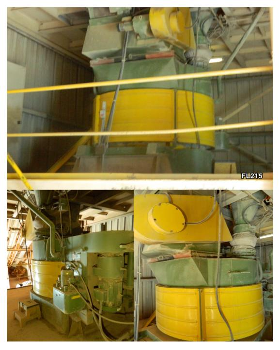
Batch capacity approximately 800 kg. Mixing pan driven by 22 kw motor and the high duty agitator powered by a 37 kw drive. Hydraulic operated, bottom discharge door. mixer is lined with replaceable wear parts. Commissioned in 1992.
