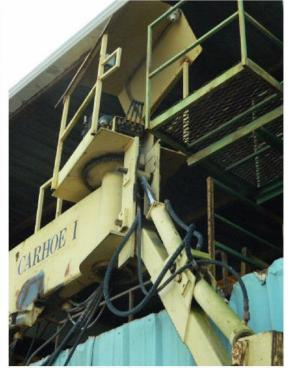
Hydraulic operated, multi-directional boom designed to aid in efficiently unloading open top, bottom dump railcars. Especially effective when unloading all types of clay, even wet. Eliminates the need for laborers inside the car, reducing labor and increasing safety. Asking price \$6,500.
