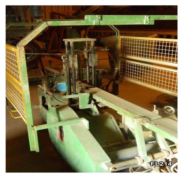
Can cut clay column up to 2.5" wide and 13" high with a self cleaning wire. Maximum cut length is 13 inches. Cuts up to 60 cuts/minute for sizes 4x8 to 12x12. Cuts are controlled electronically with encoded DC drive. Electric control panel included. Pneumatic pre-grooving for products such as split tile. Commissioned in 1992. Asking \$17,500 (original price DM 131,500).
