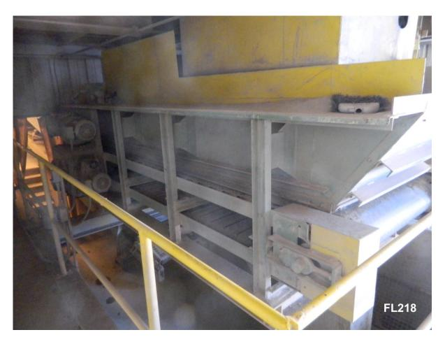
3.5 meter proportioning belt, discharge opening 1250 x 600 mm. Paddle shaft at discharge for material metering. Rubber belt bolted-on to slats that are chain and sprocket driven. Variable speed, approximately 3.4-19.4 cubic meters/hour. Overall length 4.4 meters.
