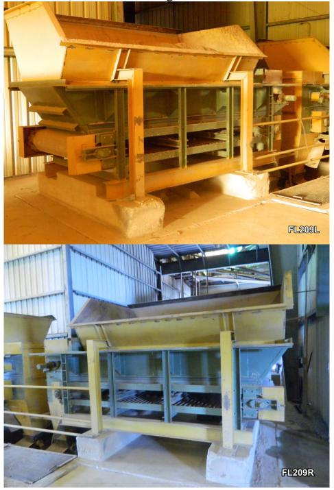
Rubber belt feeder with 3.5 meter(a.c.) proportioning belt, discharge opening 1250 x 600 mm. Paddle shaft at discharge for material metering. Rubber belt bolted-on to slats that are chain and sprocket driven. Variable speed, approximately 3.4-19.4 cubic meters/hour. Overall length 4.4 meters. Two available- 1 left hand drive, 1 right hand drive
