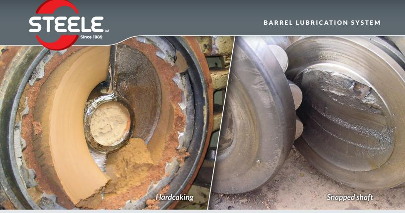
Better barrel lubrication helps prevent component failure.
