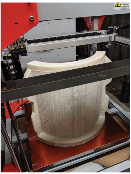
JC Steele's pattern makers devised a solution by applying traditional techniques used in patterning with mahogany to 3D printed plastic parts.
