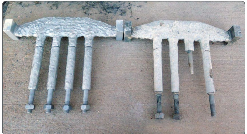
A new coated bridge (left), ready to replace worn bridge, with 30 million-plus brick on it, at right.
