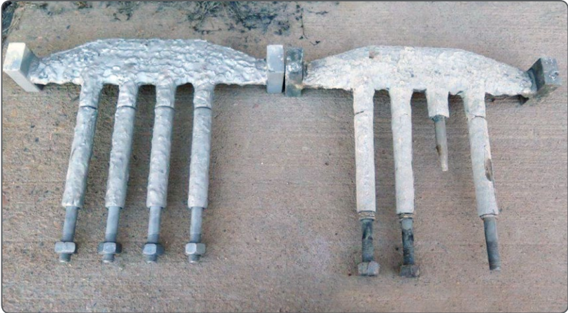
A new coated bridge on the left, ready to replace the worn bridge with 30 million-plus bricks on it, at right.
