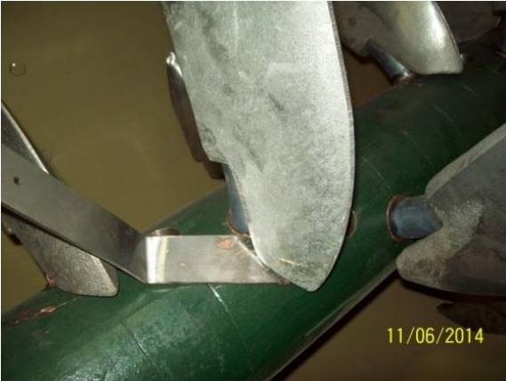
FIG 11: Using a spacer to tighten the bolt
