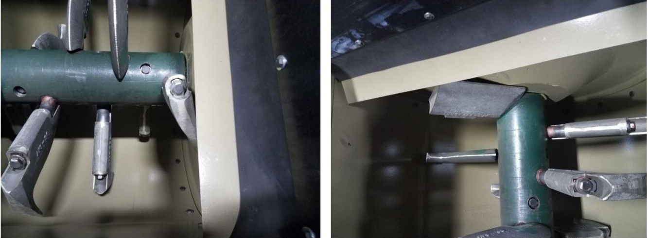
FIG 15 & 16: Photos of a properly installed rear pug knife
